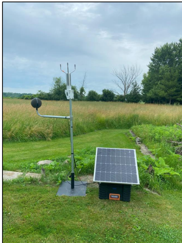
Figure 4-1. Representative Sound Monitoring Setup
